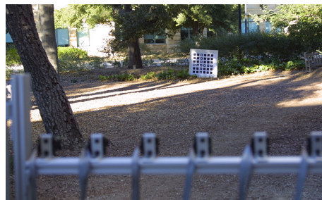
Figure 4.2: Outdoor synthetic aperture imaging setup. (a) Experimental setup showing scene layout and distances in meters from camera array. The calibration volume is the region over which the calibration grid was moved. (b) Our 45 camera array on a mobile cart. The array was controlled by a standalone 933 MHz Linux PC. (c) The view from behind the camera array showing our calibration target in front of the bushes. Our goal was to try and see people behind the bushes.
