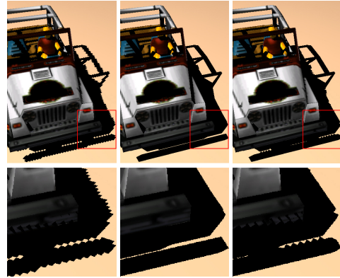
Figure 8: A closeup reveals artifacts of our algorithm when the resolution of the silhouette map is too low. (Left) standard shadow map and associated artifacts. (Center) Shadow volumes yields correct shadow. (Right) Silhouette map at the same resolution as the shadow map shows artifacts. In this case, the fender of the jeep yields an artifact like that in the center diagram of Figure 7.
