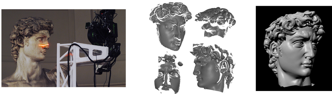
Figure 1.3: Range image registration. Left: a scan is acquired from a single viewpoint. Middle: To cover the entire object, multiple viewpoints are necessary. Right: views registered into final model. (Images courtesy Digital Michelangelo Project [58])
