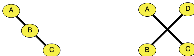
Figure 5.3: Traditional layouts avoid crossings to prevent false attachments. Left: Node-edge crossings lead to ambiguity, where it is not clear if A is connected to C and B is merely in the way, or if A and B are connected as are B and C. Right: Edge-edge crossings create visually salient “X” artifacts that draw the viewer’s attention from the important aspects of the graph structure.
