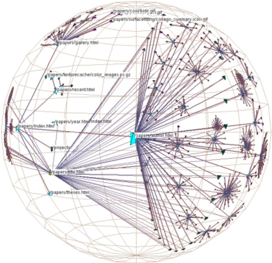
Figure 3.20: Part of the Stanford graphics group web site drawn as a graph in 3D hyperbolic space. The entire site has over 14,000 nodes and 29,000 edges. About 4000 nodes in a 7-hop diameter neighborhood of the papers archive are visible in this snapshot. One dozen of the nodes are labelled, a few hundred more have visible color coding or are individually distinguishable, and the rest of the nodes on the fringe provide aggregate information about their presence or absence. In addition to the main spanning tree, we draw the nontree outgoing links from an index of every paper by title. The tree is oriented so that ancestors of a node appear on the left and its descendants grow to the right.
