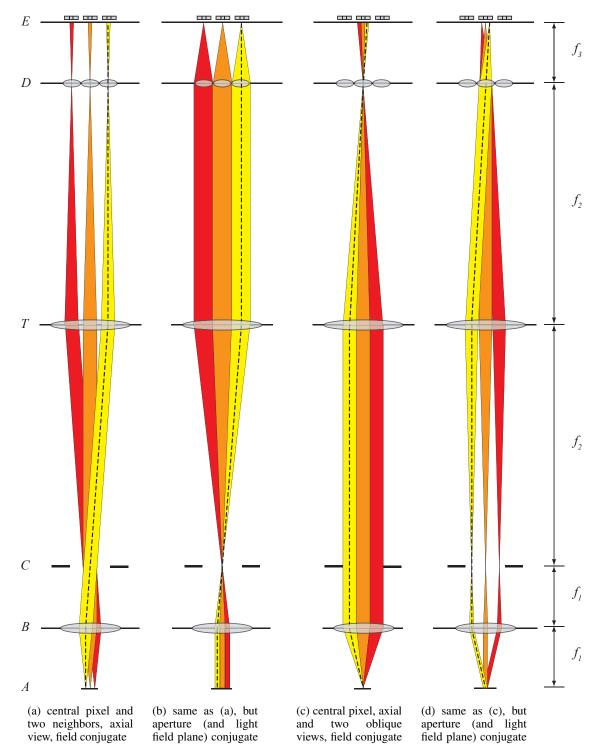
Case 2: infinity-corrected optics. The specimen A is imaged by an objective B through a telecentric stop C and a tube lens T onto intermediate image plane D. A microlens array placed at D forms multiple subimages on sensor plane E. Three such subimages are shown, as before.
