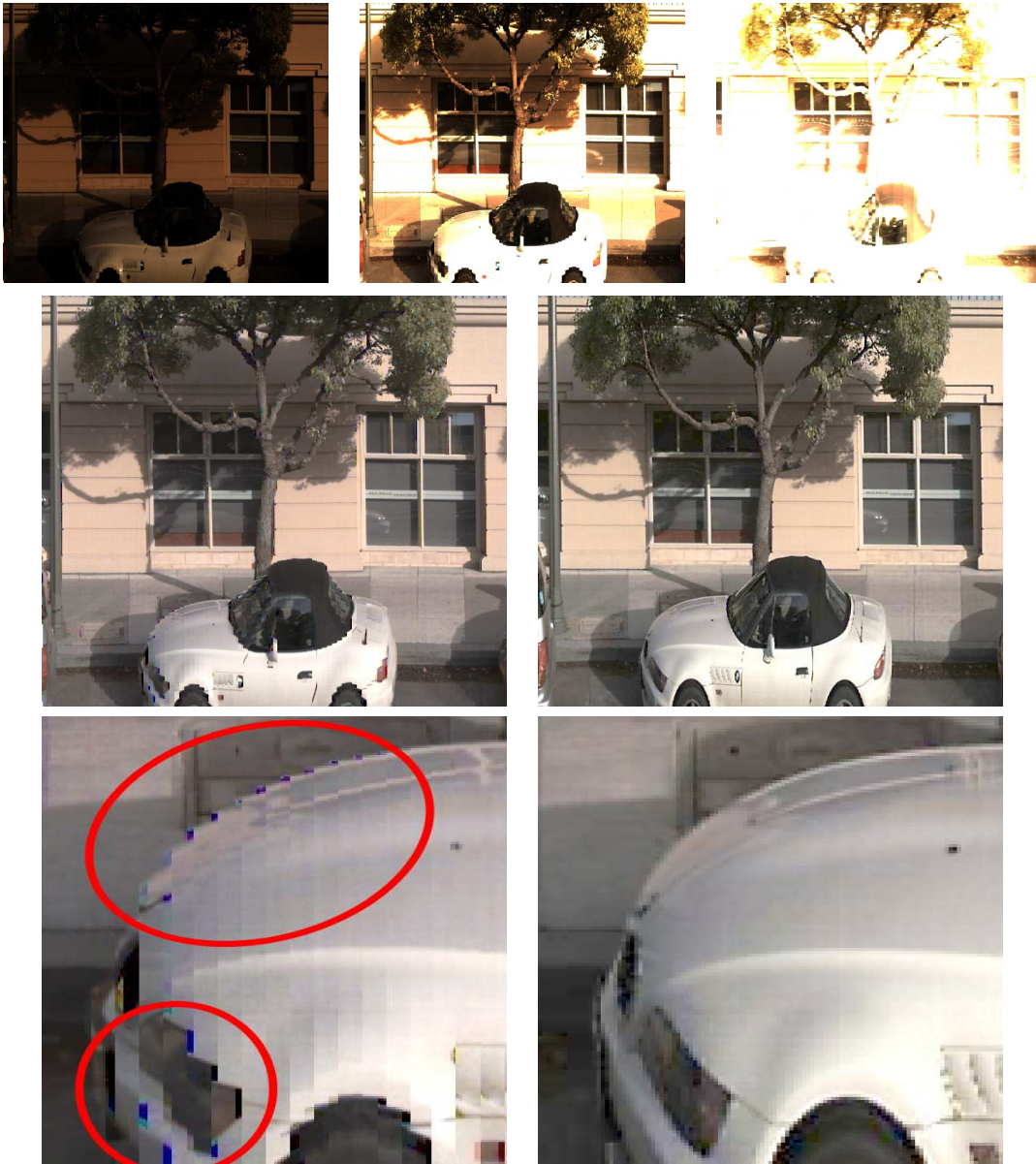
Figure 4.6: An example of the high-dynamic range assembly, including the effects of optical flow. This example shows a crop of a brighter area of the street, in contrast to the darker section shown in Figure 4.5. (top row) A segment of the multiperspective images rendered at each of three exposures. (middle left) The same segment after combining the three low-dynamic range images and tone-mapping using a gamma curve, without optical flow. (middle right) The same region after rendering the three segments using optical flow and then combining them. (bottom row) Zoom of middle row. Notice the lack of color artifacts on the front edge of the car.
