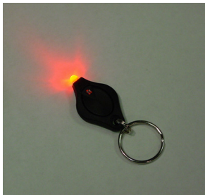
Figure 5 A bright LED used as a feature easily identifiable in both a tracking system and by the pan-tilt cameras.
