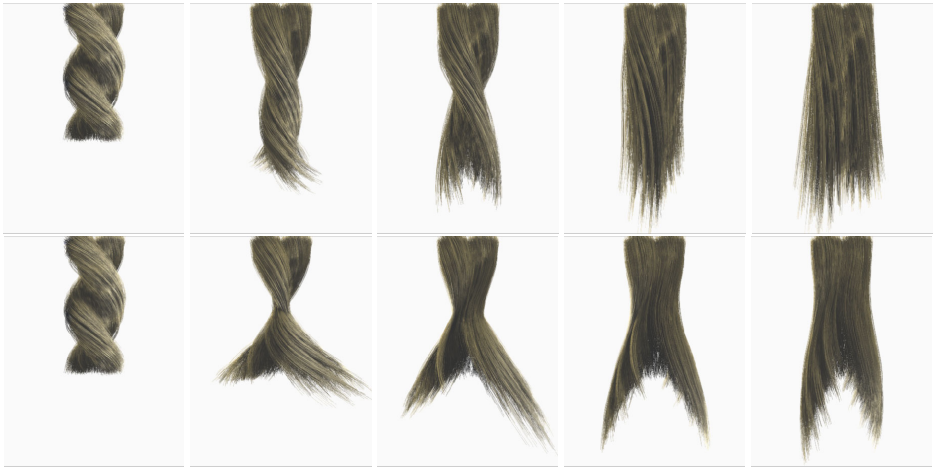
Figure 14: A comparison between two hair animations with and without collision detection. Top row: braided hair unfolds correctly in a spiral motion because of the collision detection. Bottom row: hairs penetrate each other when there is no collision detection.
